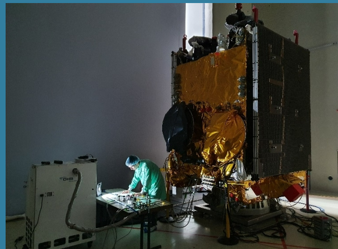
H2Sat ( GEO telecom sat from OHB System) Xenon Loading by OHB Sweden using inhouse developed Xenon Loading Cart. OHB Sweden is responsible for the entire EP-system.
